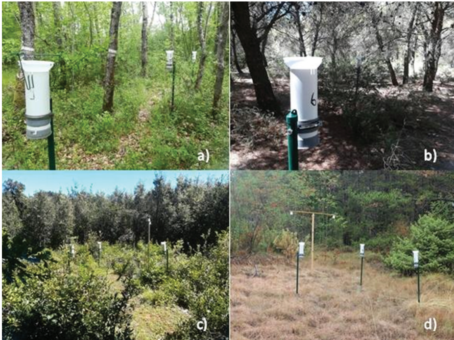
Figure 2. Collectors for throughfall deposition (THR) in (a) pubescent oak (PO) and (b) Aleppo pine (AP) and bulk deposition (BOF) in (c) holm oak (HO) and (d) black pine (BP).
